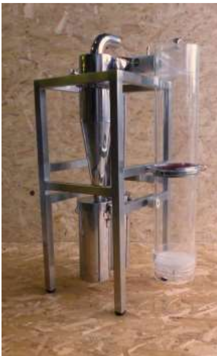
cyclone and substrate column
