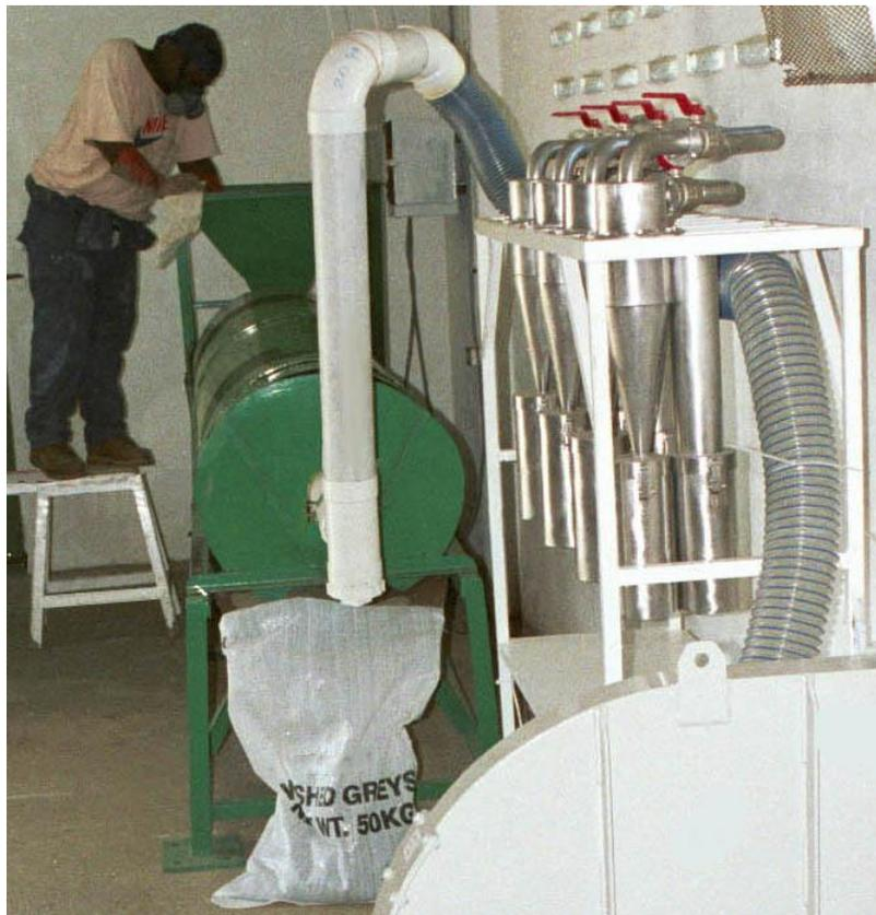
**Process:** The substrate agitator is a continuous process. The advantage of having 4 (or more) cyclones is that they can be shut off individually for removal of conidia, without shutting down the rest of the process.
